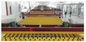
With a length of approximately 190m, the cold end equipment from Grenzebach is the end of the latest float glass production line at Gold Glass. Shown here is the main line course towards the continuous ribbon area.
